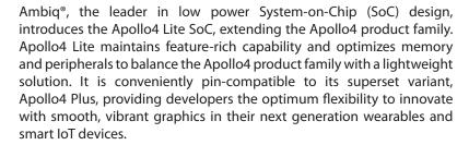
The Apollo4 Lite SoC is built upon Ambiq's proprietary Subthreshold Power-Optimized Technology (SPOT®) platform. The Apollo4 Lite complete hardware and software solution enables the battery-powered endpoint devices of tomorrow to achieve a higher level of intelligence without sacrificing battery life. The Apollo4 Lite includes a 32-bit Arm® Cortex®-M4 core with Floating Point Unit embedded in a BGA package.
