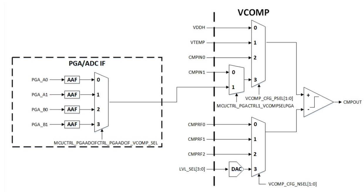
Figure 47. Block diagram for the Voltage Comparator Module
