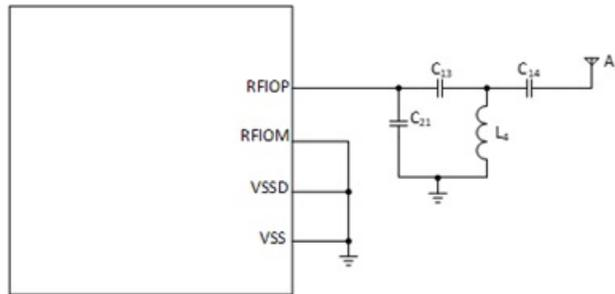
**Figure 20. Recommended Antenna Filter**
