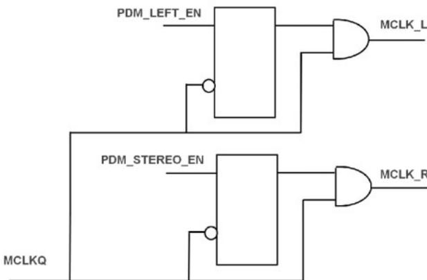
Figure 45. PDM Converter Core Local Clock Gating
