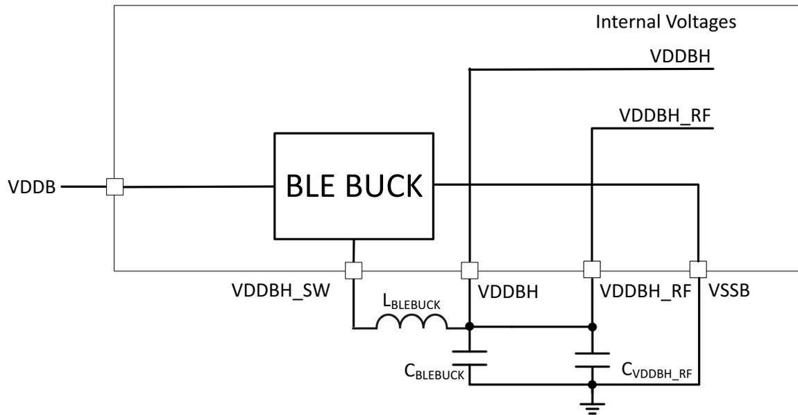
Figure 52. External Components for BLE Buck
