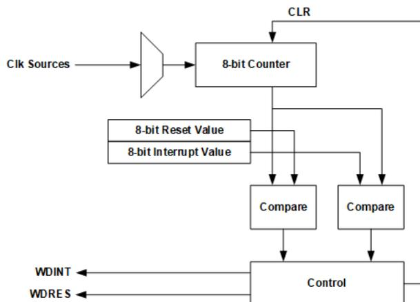
**Figure 23. Block Diagram for the Watchdog Timer Module**
