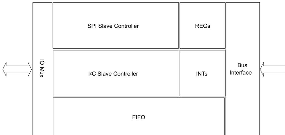
**Figure 36. Block diagram for the I<sup>2</sup>C/SPI Slave Module**
