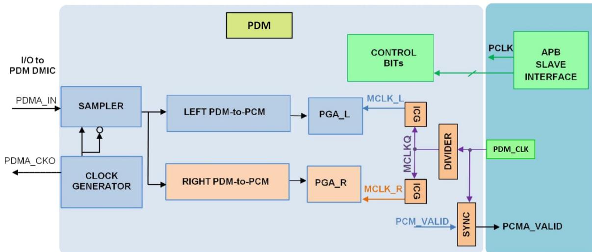
Figure 44. Clock Path and Data Synchronization Diagram
