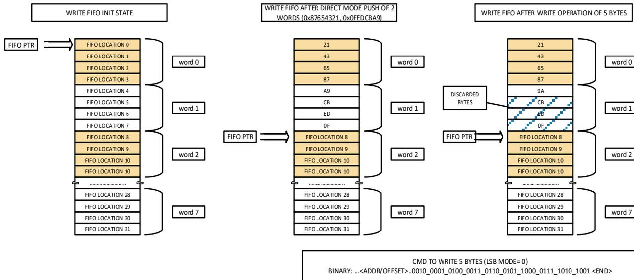
Figure 31. Direct Mode 5-byte Write Transfer
