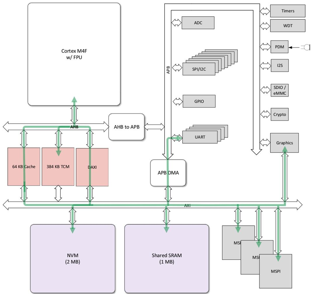
**Figure 10. Apollo4 Blue Lite SoC System Diagram**
