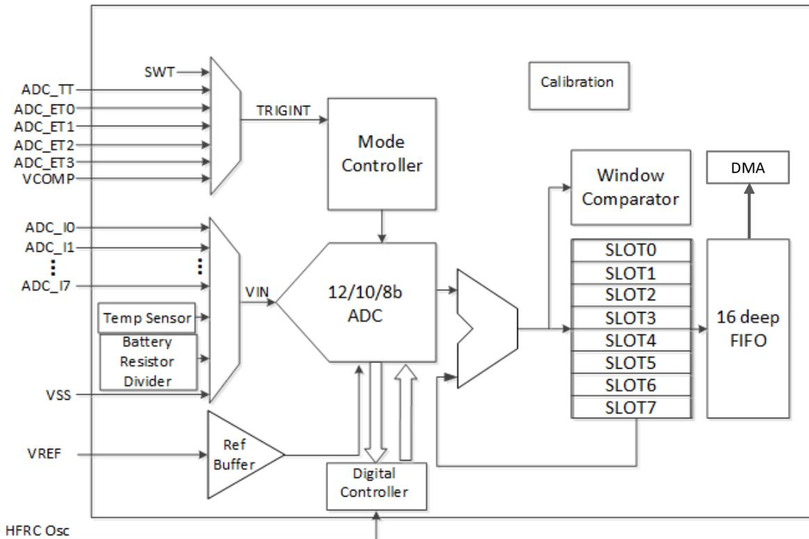
Figure 25. Block Diagram for ADC and Temperature Sensor
