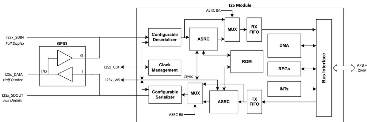
Figure 46. I<sup>2</sup>S Block Diagram
