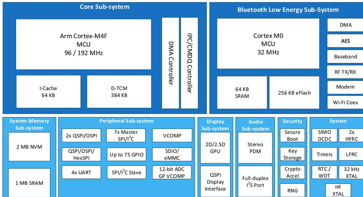
**Figure 2. Apollo4 Blue Lite SoC Block Diagram**
