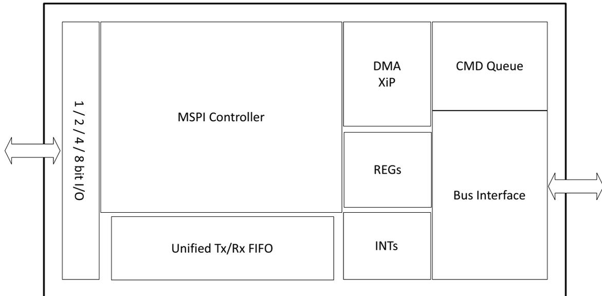
Figure 27. Block Diagram for the MSPI Master Module
