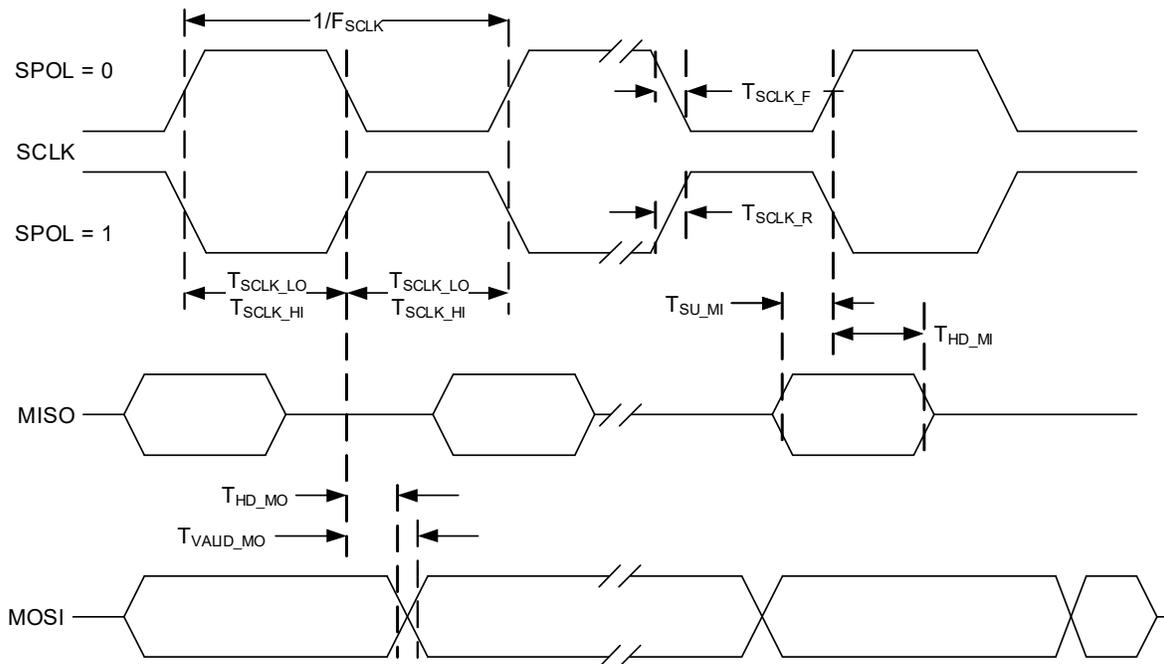
Figure 53. SPI Master Mode, Phase = 0
