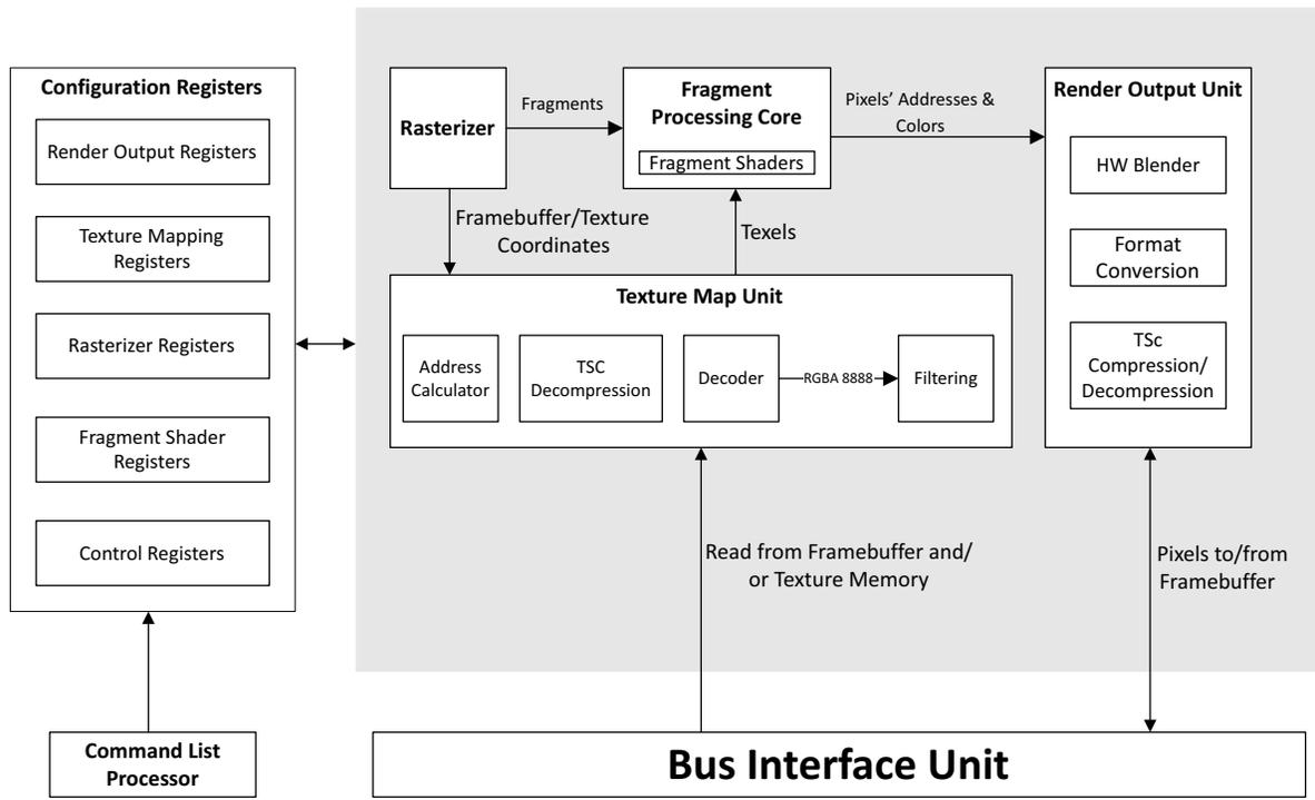
Figure 39. GPU Block Diagram
