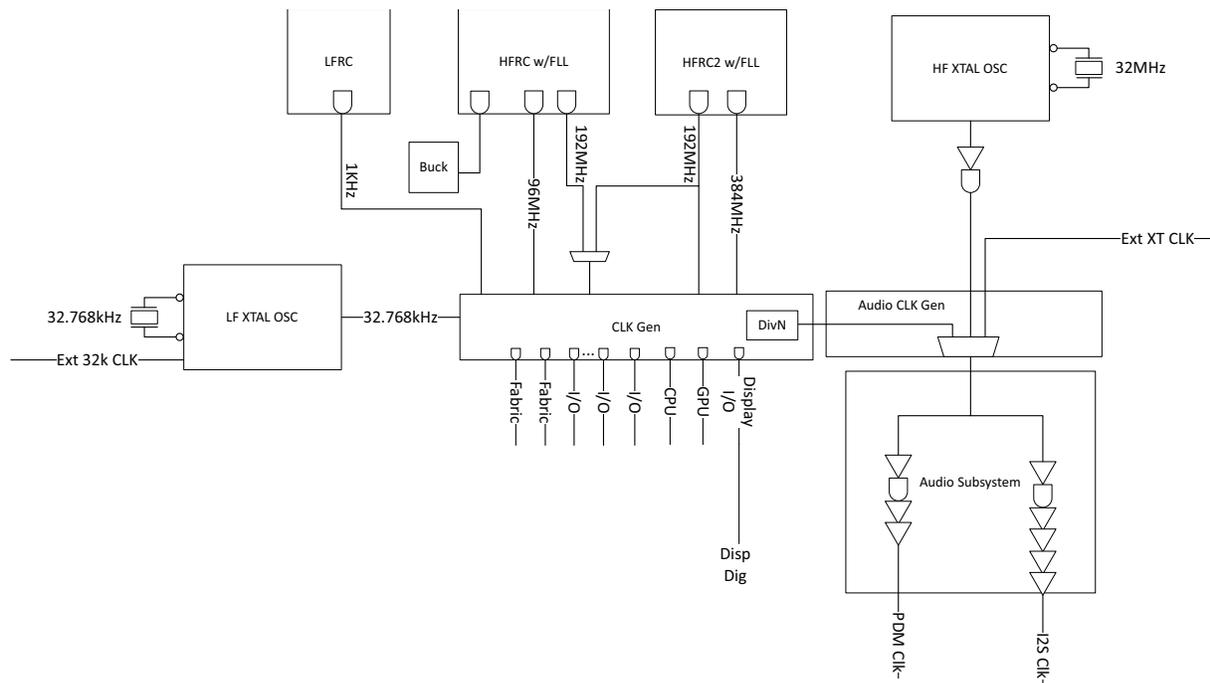
Figure 13. Block diagram for the Clock Generator
