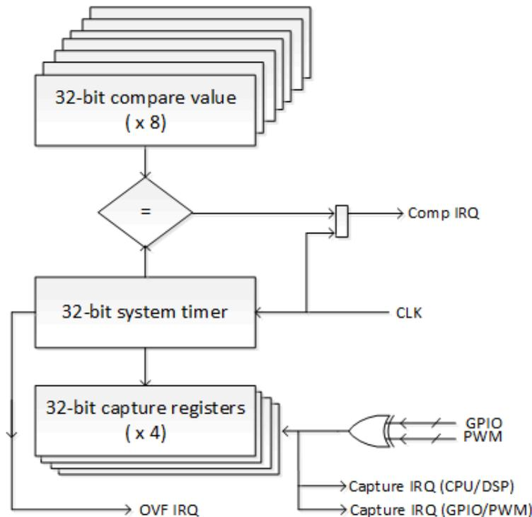
**Figure 22. Block Diagram for the System Timer**
