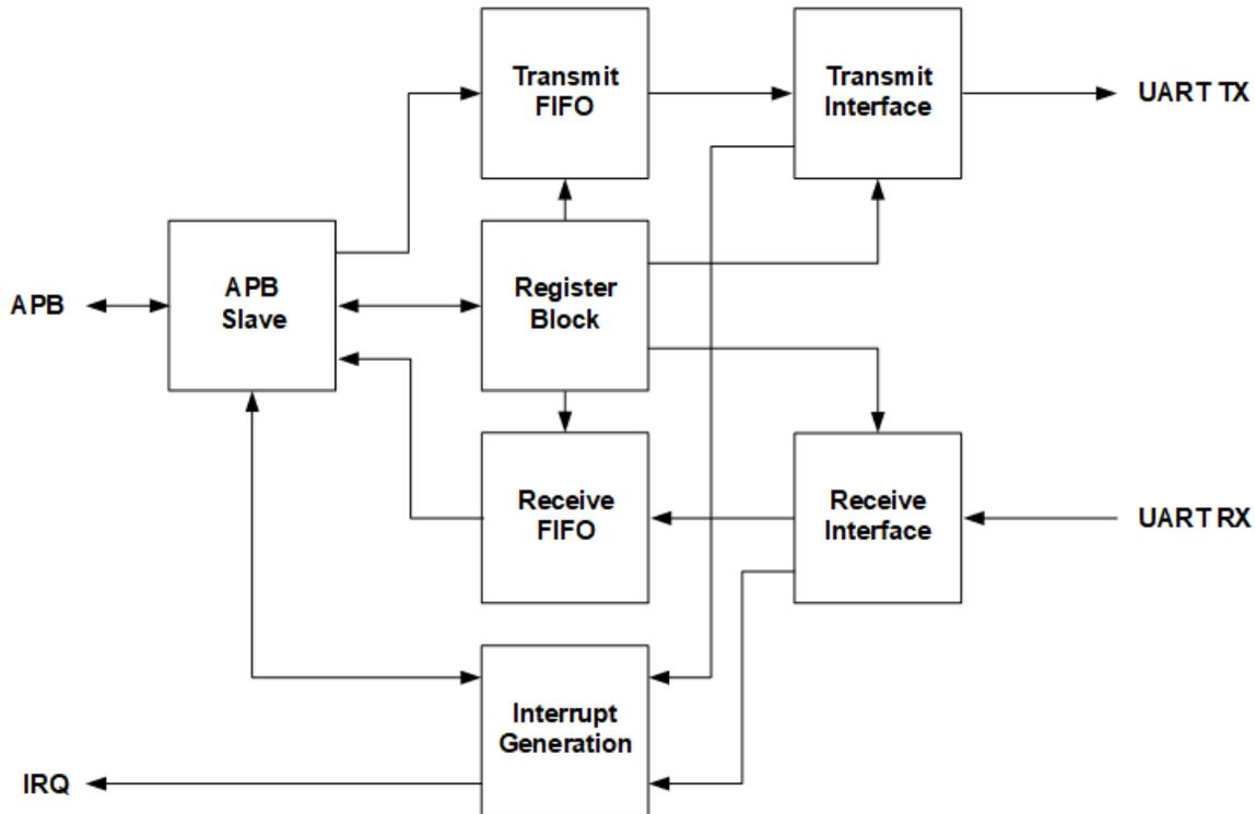
Figure 37. Block Diagram for the UART Module
