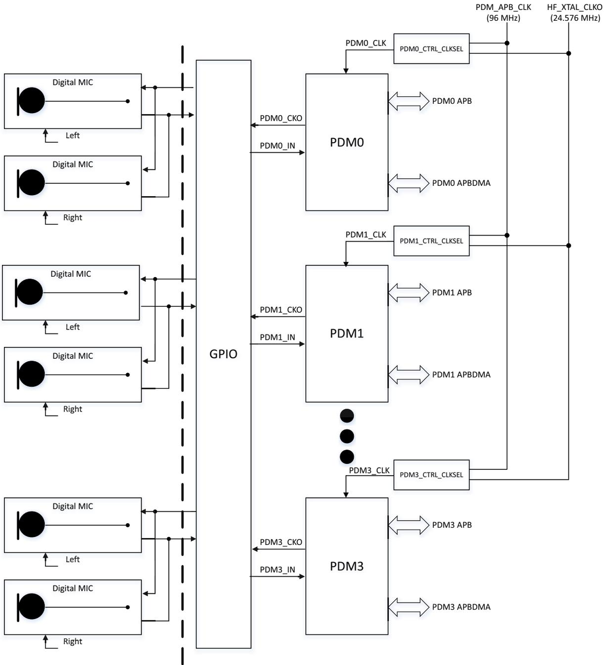
Figure 42. PDM Instances within Audio Subsystem (4 PDMs Shown)
