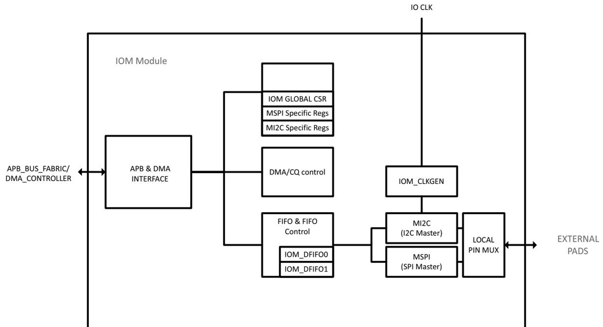
Figure 28. Block Diagram for the I<sup>2</sup>C/SPI Master Module
