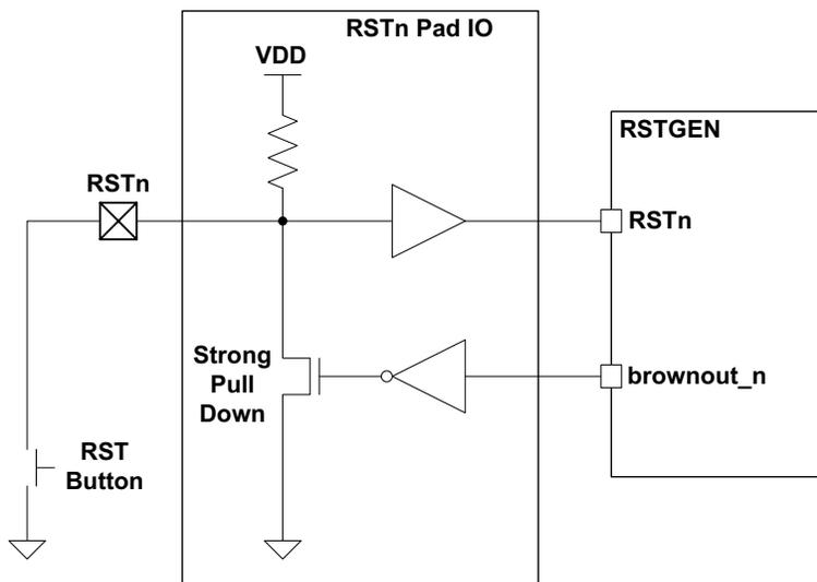
Figure 12. Block diagram of circuitry for Reset pin
