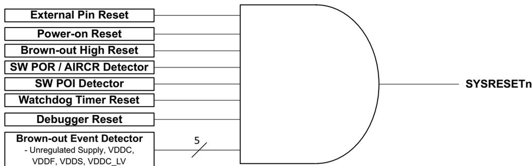
Figure 11. Block diagram for the Reset Generator Module
