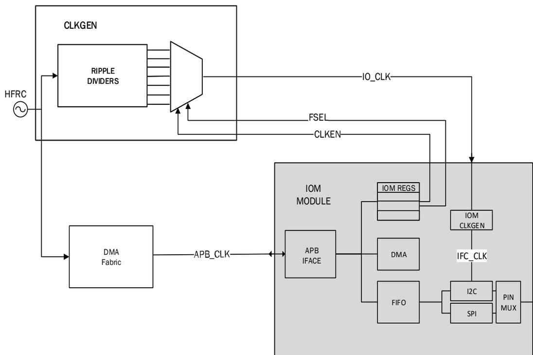
**Figure 29. Clocking Structure for IOM Module**
