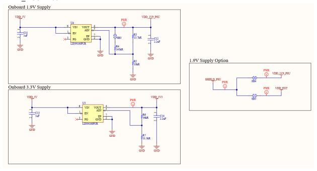
Figure 4. PSU page of the Display Shield schematic
