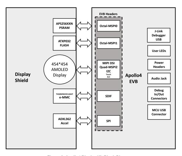
Figure 2. Apollo4 Display Kit Block Diagram
