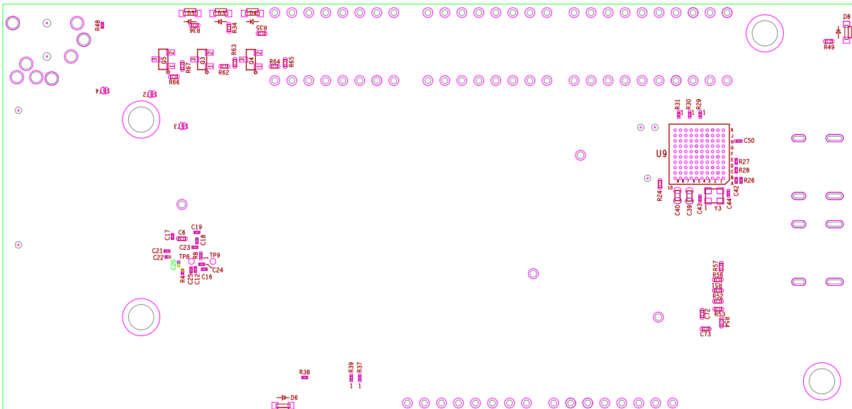
Figure 4. Apollo4 Blue EVB - Bottom-side Parts Location
