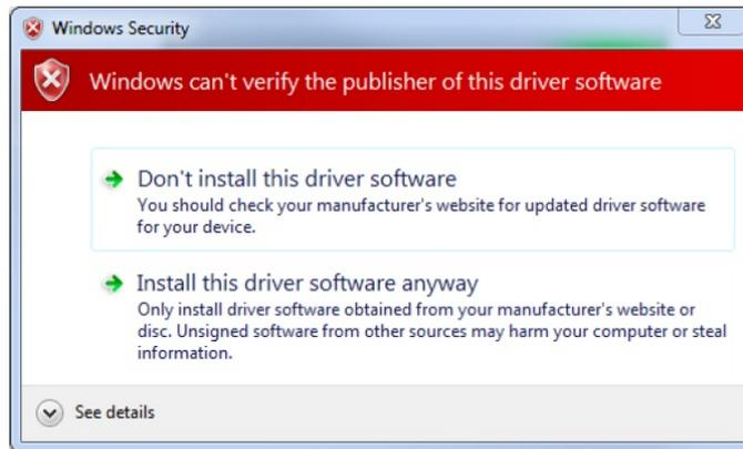
A window will indicate if the installation is successful. Repeat this process for each of the USB interfaces with missing drivers. After this is complete, the Ambiq debugger tools should be able to connect to the Apollo EVK correctly.
