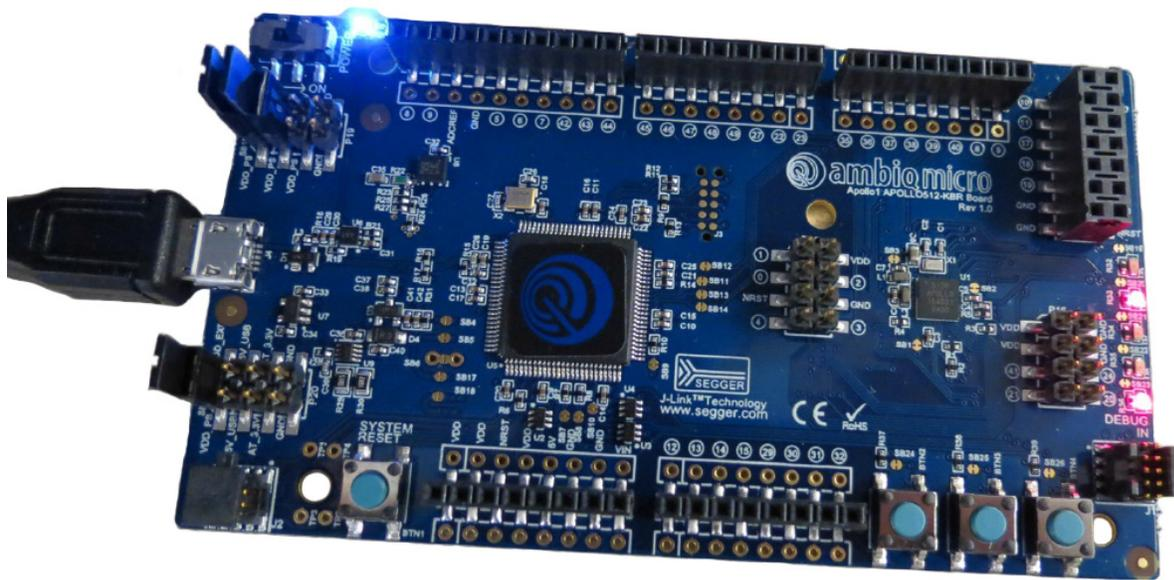
The debug interface is supported by standard J-Link drivers from Segger. Refer to *Section 4 Software Development Tools for the Apollo EVB* on page 9 for more details on J-Link debug support.
